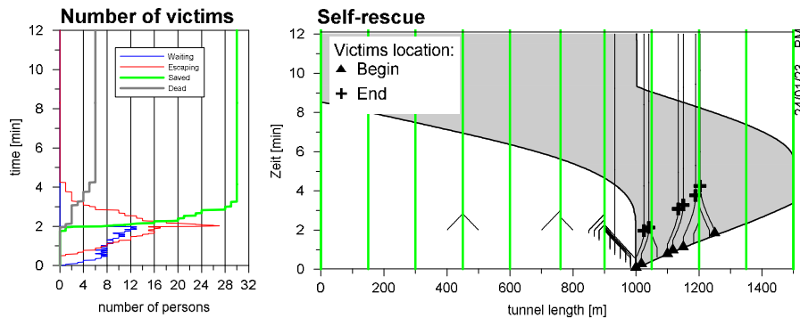
Figure 6. Natural ventilation, emergency exits every 150 m - Person position in time (right) and self-rescue evolution (left).
