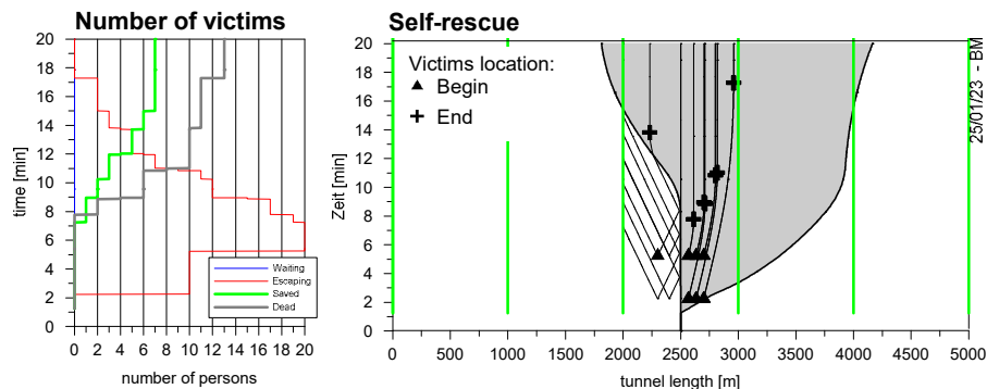
Figure 10. Person position in time (right) and self-rescue evolution (left) – Emergency exits ever 1000 m.
