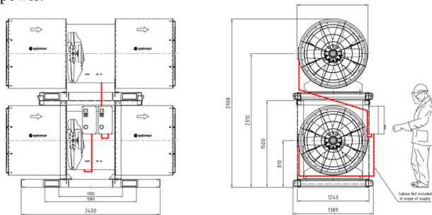
Figure 12 Jet fans for supporting natural ventilation
