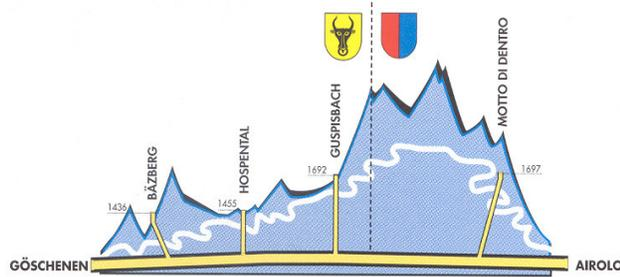
Figure 6 Schematic representation of the 17 km Gotthard Road tunnel with 4 high shafts (Bettelini, 2004)
