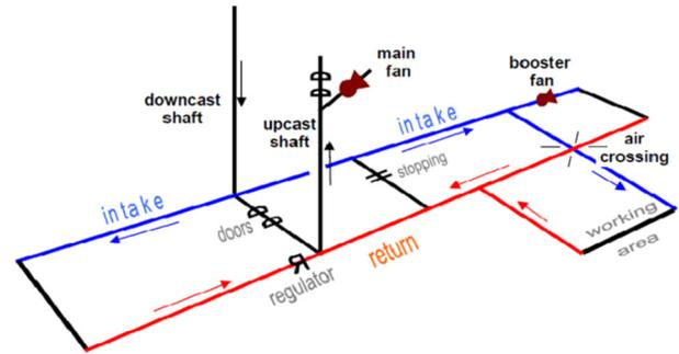
Figure 4 Schematic representation of the Okaba Underground Coal Mine (Nigeria) ventilation system (Akande and Moshood, 2013)
