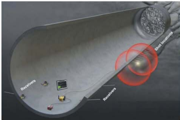
Figure 1. Schematic visualisation of a standard TSP layout in conventional tunnelling.
