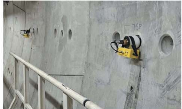
Figure 2. Two TSP 603 wireless transceivers attached to TSP receivers deployed 1.5 m deep in boreholes through the grout hole of precast segments.
