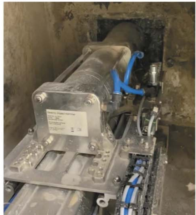
Figure 3. Controlled impact hammer of TSP-Impact. The impact cylinder, in which the impact mass is accelerated, is coupled to the lateral rock wall through an opening in the TBM's shield shell by the feed cylinder below.
